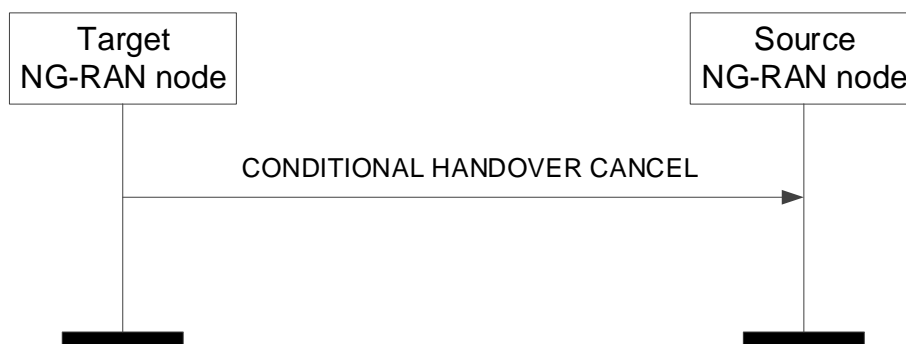
Figure 8.2.9.2-1: Conditional Handover Cancel, successful operation
