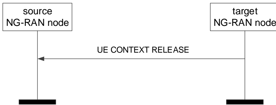
Figure 8.2.7.2-1: UE Context Release, successful operation for handover
