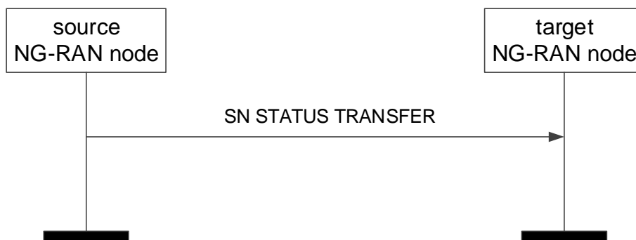
Figure 8.2.2.2-1: SN Status Transfer, successful operation
