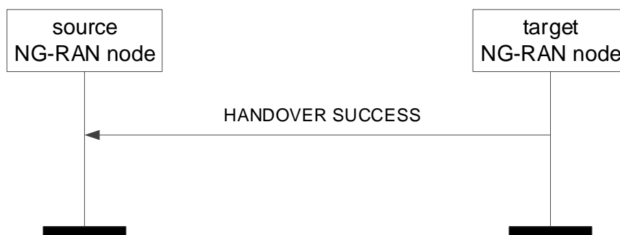
Figure 8.2.8.2-1: Handover Success, successful operation
