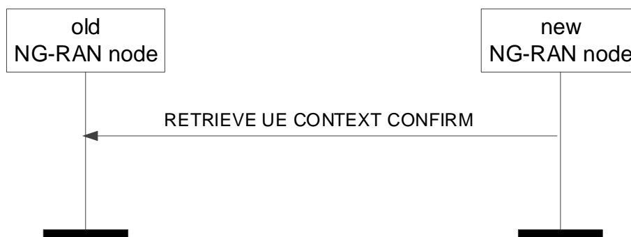
Figure 8.2.12.2-1: Retrieve UE Context Confirm, successful operation
