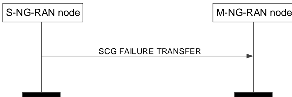
Figure 8.3.18.2-1: SCG Failure Information Transfer, successful operation
