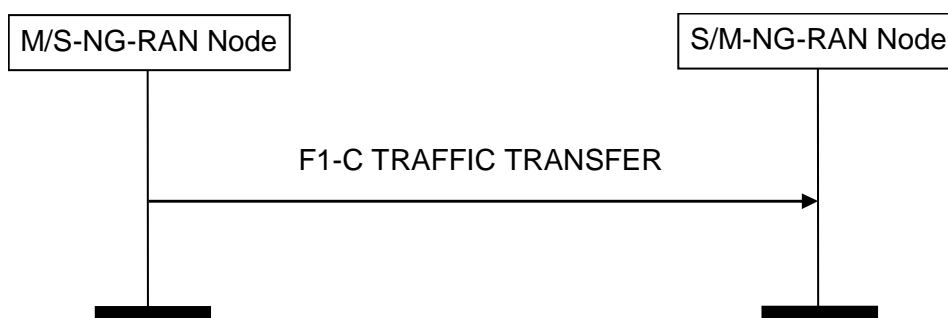
Figure 8.5.1.2-1: F1-C Traffic Transfer procedure, successful operation
