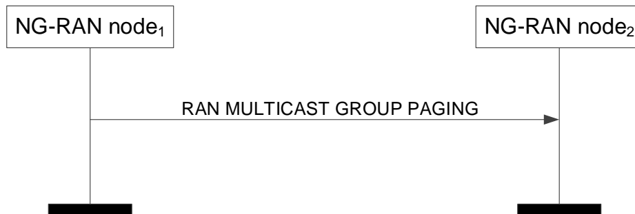
Figure 8.2.11.2-1: RAN Multicast Group Paging, successful operation
