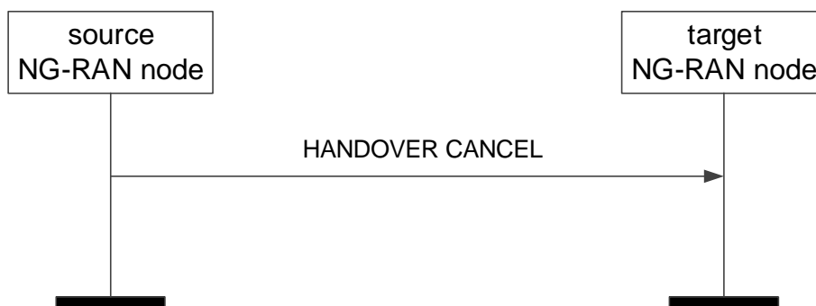
Figure 8.2.3.2-1: Handover Cancel, successful operation
