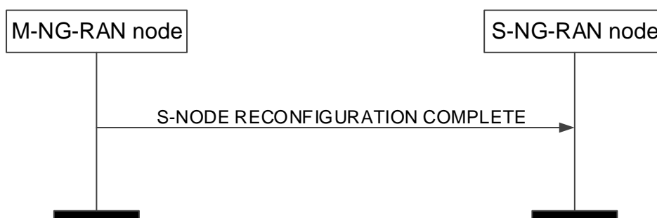
Figure 8.3.2.2-1: S-NG-RAN node Reconfiguration Complete procedure, successful operation.
