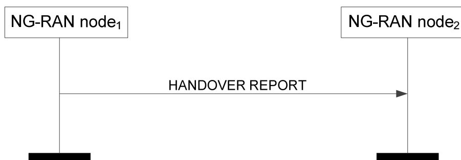
Figure 8.4.8.2-1: Handover Report, successful operation
