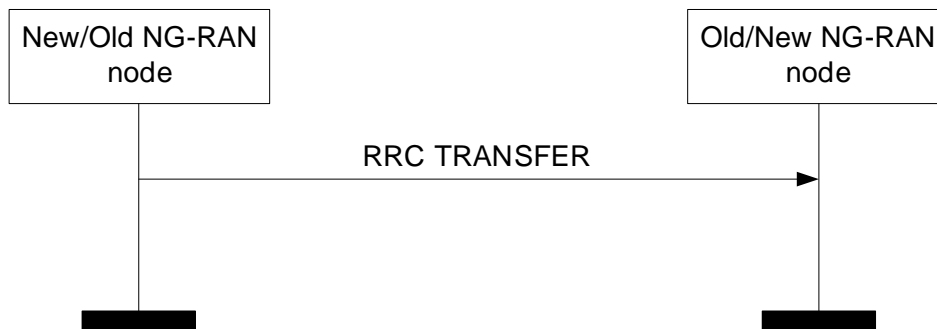
Figure 8.3.9.2-2: RRC Transfer procedure for SDT, successful operation.
