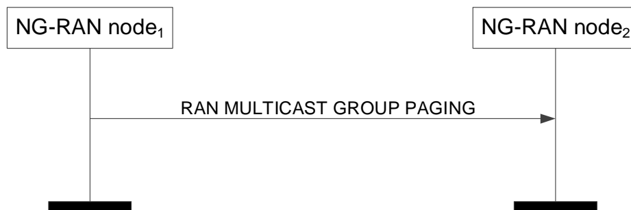
Figure 8.2.11.2-1: RAN Multicast Group Paging, successful operation
