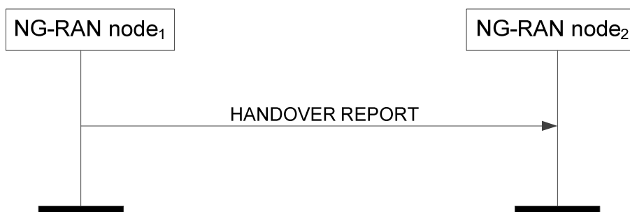
Figure 8.4.8.2-1: Handover Report, successful operation
