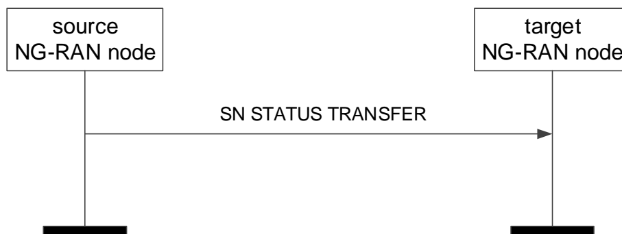
Figure 8.2.2.2-1: SN Status Transfer, successful operation
