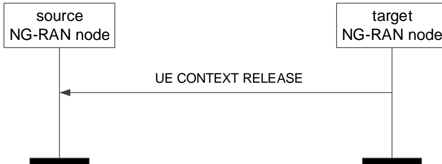
Figure 8.2.7.2-1: UE Context Release, successful operation for handover
