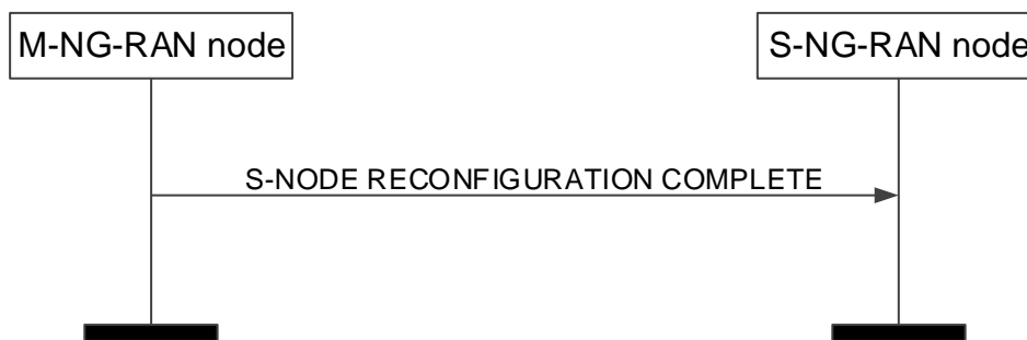
Figure 8.3.2.2-1: S-NG-RAN node Reconfiguration Complete procedure, successful operation.
