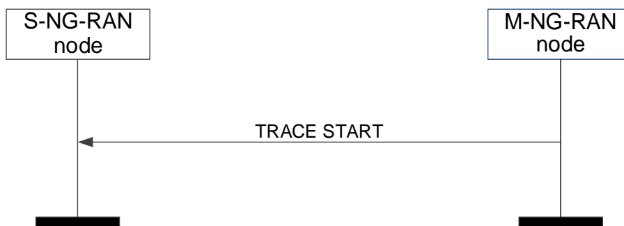
Figure 8.3.14.2-1: Trace Start, successful operation
