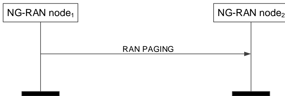
Figure 8.2.5.2-1: RAN Paging: successful operation
