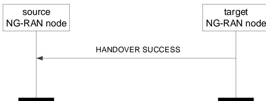
Figure 8.2.8.2-1: Handover Success, successful operation
