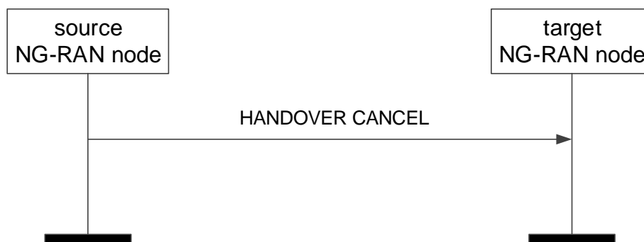
Figure 8.2.3.2-1: Handover Cancel, successful operation
