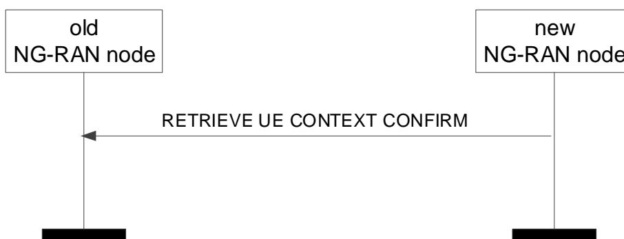
Figure 8.2.12.2-1: Retrieve UE Context Confirm, successful operation
