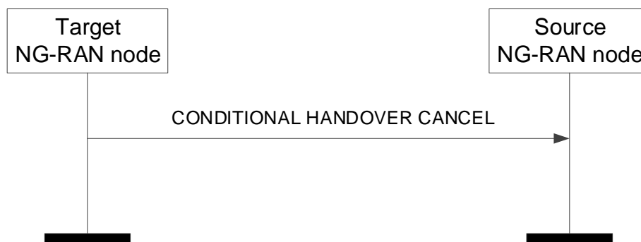
Figure 8.2.9.2-1: Conditional Handover Cancel, successful operation
