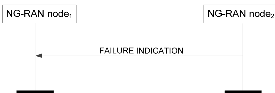
Figure 8.4.7.2-1: Failure Indication, successful operation
