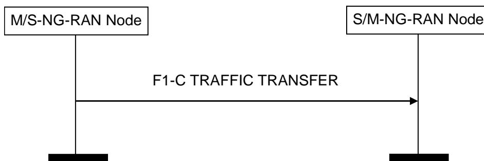
Figure 8.5.1.2-1: F1-C Traffic Transfer procedure, successful operation
