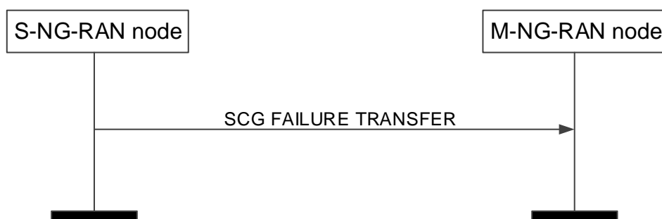
Figure 8.3.18.2-1: SCG Failure Information Transfer, successful operation
