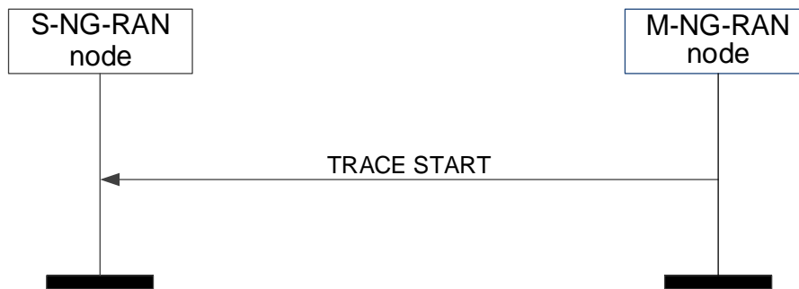
Figure 8.3.14.2-1: Trace Start, successful operation
