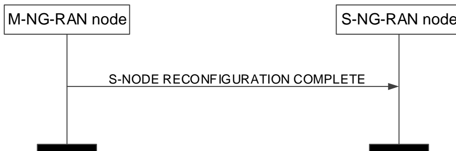
Figure 8.3.2.2-1: S-NG-RAN node Reconfiguration Complete procedure, successful operation.
