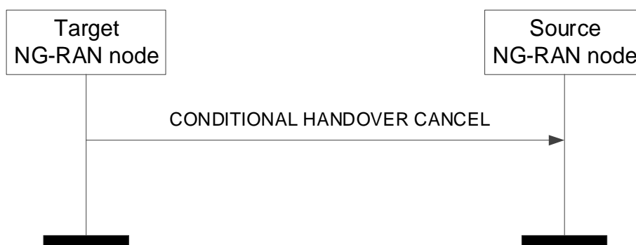
Figure 8.2.9.2-1: Conditional Handover Cancel, successful operation
