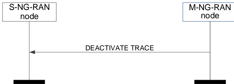
Figure 8.3.15.2-1: Deactivate Trace, successful operation
