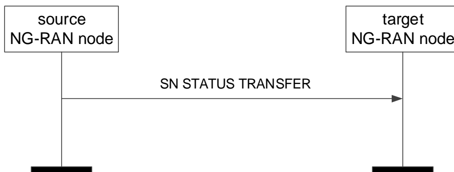
Figure 8.2.2.2-1: SN Status Transfer, successful operation
