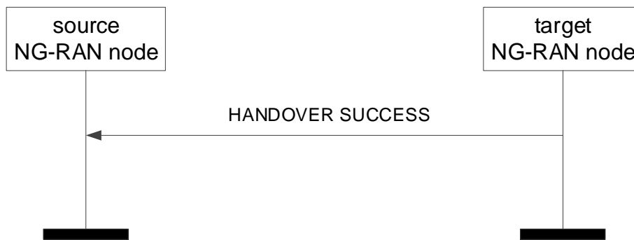
Figure 8.2.8.2-1: Handover Success, successful operation
