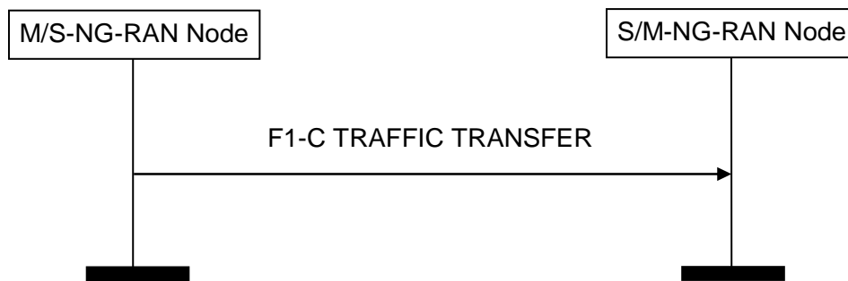
Figure 8.5.1.2-1: F1-C Traffic Transfer procedure, successful operation
