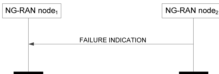
Figure 8.4.7.2-1: Failure Indication, successful operation
