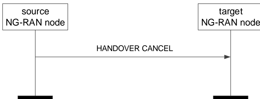
Figure 8.2.3.2-1: Handover Cancel, successful operation
