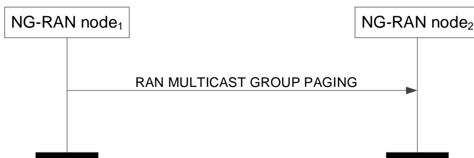
Figure 8.2.11.2-1: RAN Multicast Group Paging, successful operation
