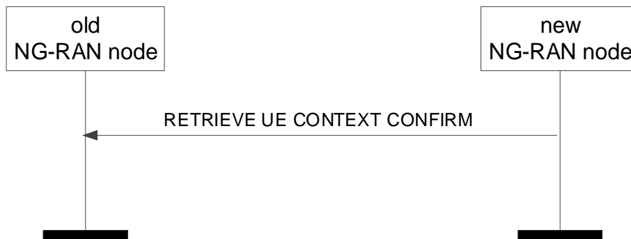
Figure 8.2.12.2-1: Retrieve UE Context Confirm, successful operation
