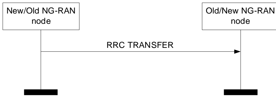
Figure 8.3.9.2-2: RRC Transfer procedure for SDT, successful operation.
