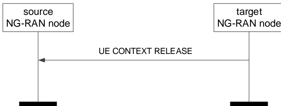
Figure 8.2.7.2-1: UE Context Release, successful operation for handover
