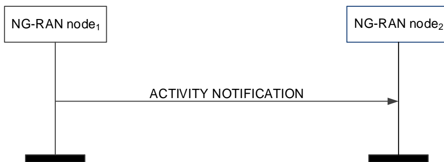
Figure 8.3.11.2-1: Activity Notification, successful operation
