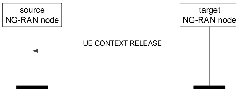
Figure 8.2.7.2-1: UE Context Release, successful operation for handover
