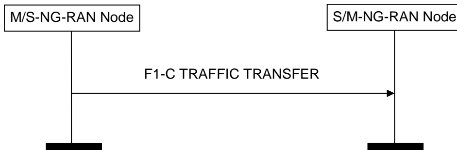
Figure 8.5.1.2-1: F1-C Traffic Transfer procedure, successful operation
