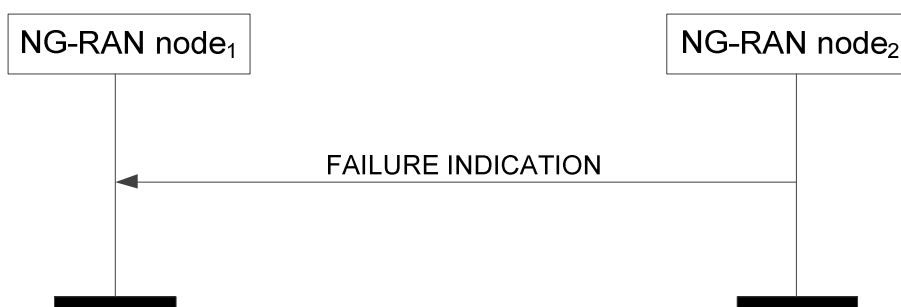
Figure 8.4.7.2-1: Failure Indication, successful operation
