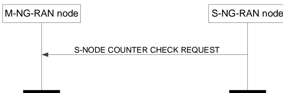
Figure 8.3.8.2-1: S-NG-RAN node Counter Check procedure, successful operation.
