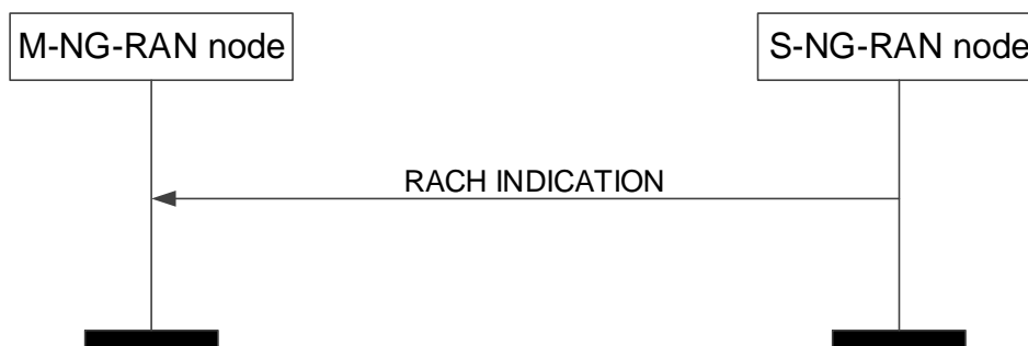
Figure 8.3.20.2-1: RACH Indication procedure, successful operation.
