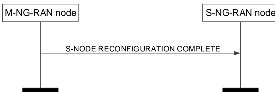
Figure 8.3.2.2-1: S-NG-RAN node Reconfiguration Complete procedure, successful operation.
