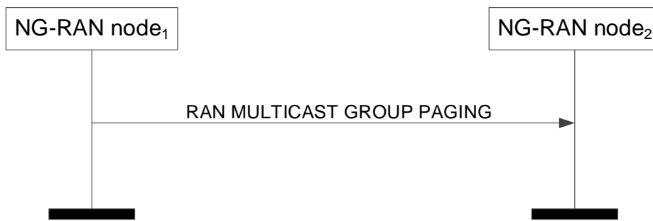
Figure 8.2.11.2-1: RAN Multicast Group Paging, successful operation
