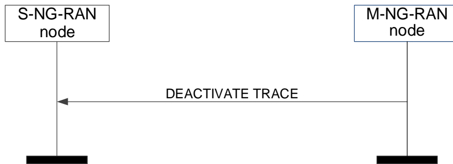
Figure 8.3.15.2-1: Deactivate Trace, successful operation
