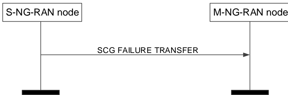
Figure 8.3.18.2-1: SCG Failure Information Transfer, successful operation
