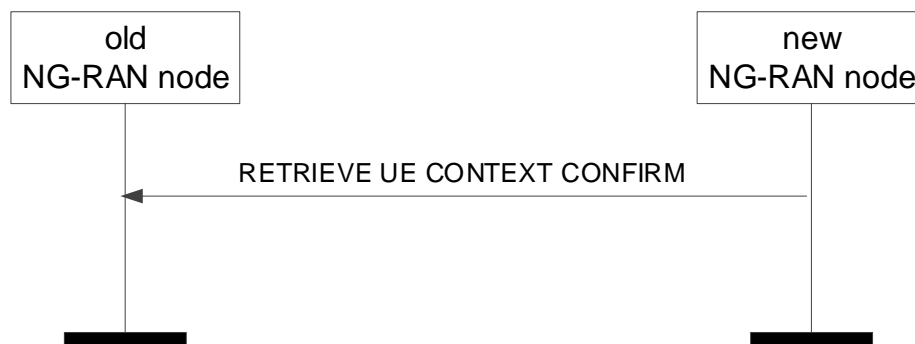
Figure 8.2.12.2-1: Retrieve UE Context Confirm, successful operation
