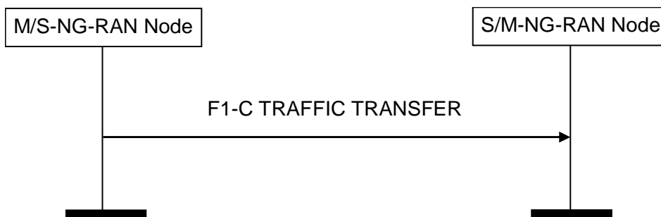
Figure 8.5.1.2-1: F1-C Traffic Transfer procedure, successful operation
