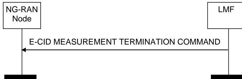
Figure 8.2.4.2-1: E-CID Measurement Termination procedure, successful operation
