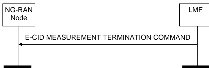
Figure 8.2.4.2-1: E-CID Measurement Termination procedure, successful operation
