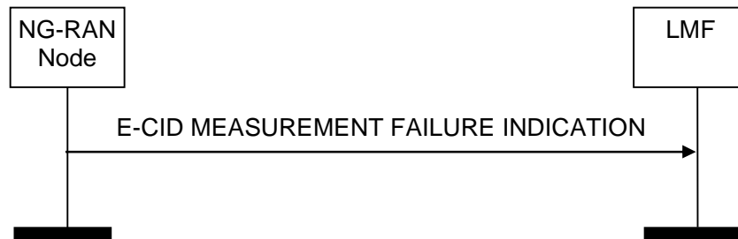
Figure 8.2.2.2-1: E-CID Measurement Failure Indication, successful operation
