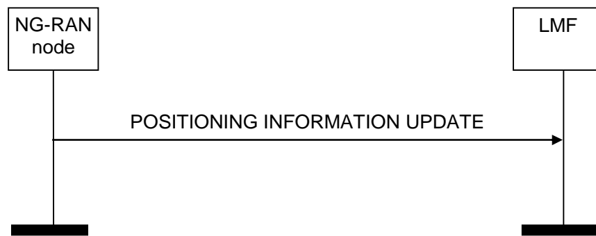
Figure 8.2.7.2-1: Positioning Information Update procedure, successful operation
