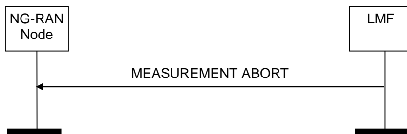
Figure 8.5.4.2.1: Measurement Abort Procedure: Successful Operation.
