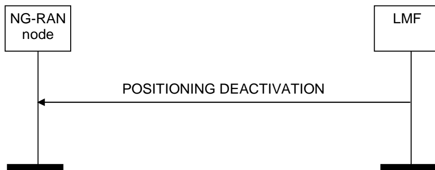
Figure 8.2.10.2-1: Positioning Deactivation procedure, successful operation
