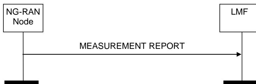
Figure 8.z.2.2.1: Measurement Report procedure. Successful operation.
