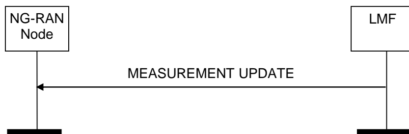
Figure 8.5.3.2.1: Measurement Update: Successful Operation.
