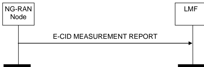
Figure 8.2.3.2-1: E-CID Measurement Report procedure, successful operation
