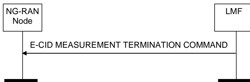
Figure 8.2.4.2-1: E-CID Measurement Termination procedure, successful operation
