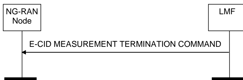
Figure 8.2.4.2-1: E-CID Measurement Termination procedure, successful operation
