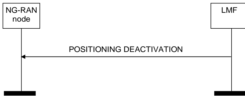
Figure 8.2.10.2-1: Positioning Deactivation procedure, successful operation
