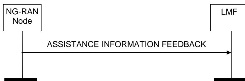
Figure 8.4.2.2-1: Assistance Information Feedback procedure
