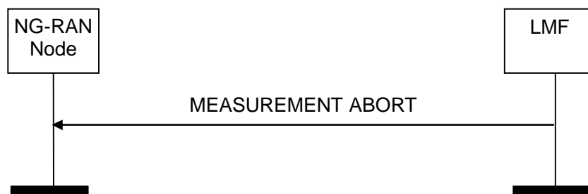
Figure 8.5.4.2.1: Measurement Abort Procedure: Successful Operation.
