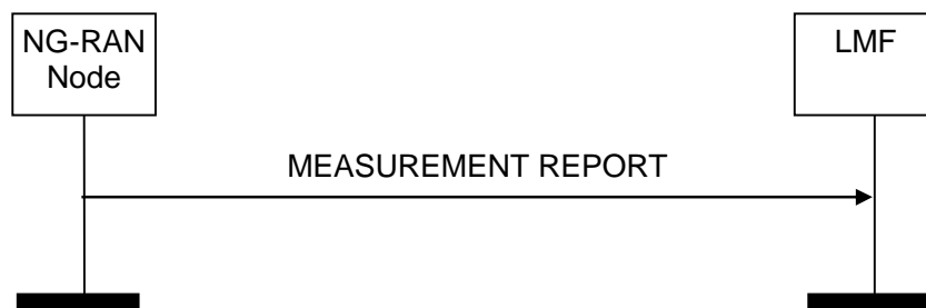
Figure 8.5.2.2.1: Measurement Report procedure. Successful operation.
