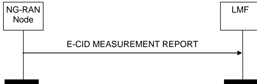
Figure 8.2.3.2-1: E-CID Measurement Report procedure, successful operation
