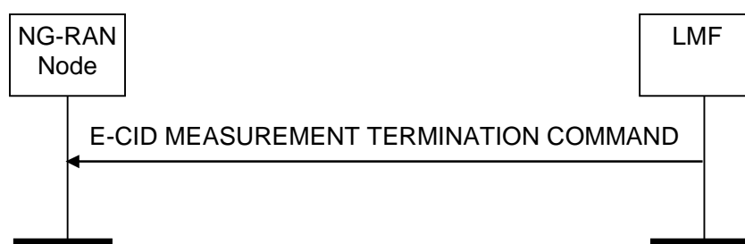
Figure 8.2.4.2-1: E-CID Measurement Termination procedure, successful operation
