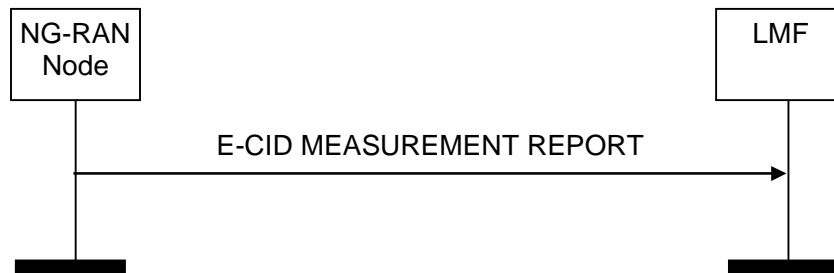
Figure 8.2.3.2-1: E-CID Measurement Report procedure, successful operation
