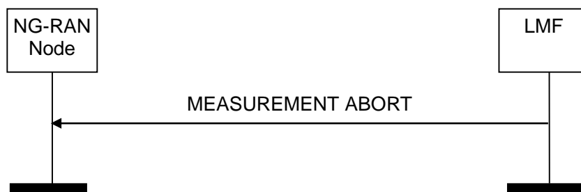
Figure 8.5.4.2.1: Measurement Abort Procedure: Successful Operation.
