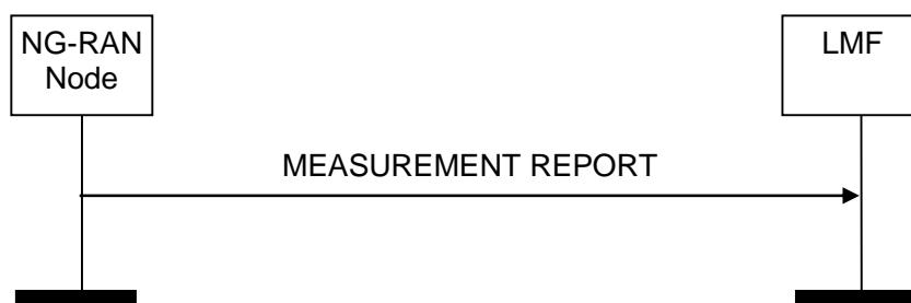
Figure 8.5.2.2.1: Measurement Report procedure. Successful operation.
