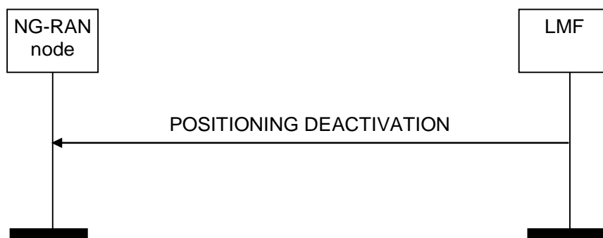
Figure 8.2.10.2-1: Positioning Deactivation procedure, successful operation
