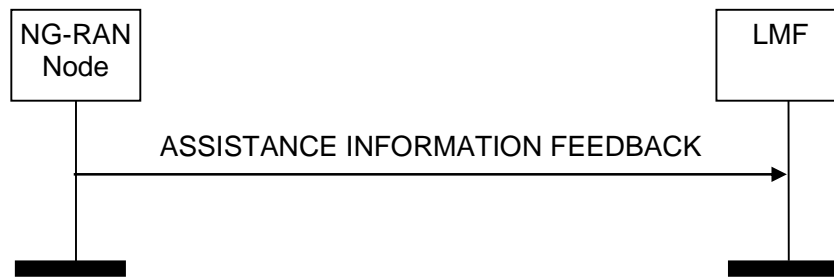
Figure 8.4.2.2-1: Assistance Information Feedback procedure
