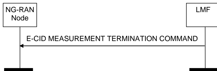
Figure 8.2.4.2-1: E-CID Measurement Termination procedure, successful operation
