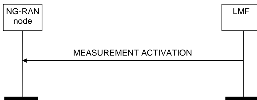
Figure 8.2.13.2-1: Measurement Activation procedure, successful operation
