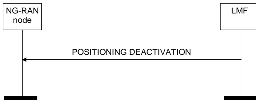
Figure 8.2.10.2-1: Positioning Deactivation procedure, successful operation
