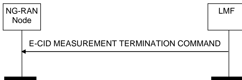
Figure 8.2.4.2-1: E-CID Measurement Termination procedure, successful operation
