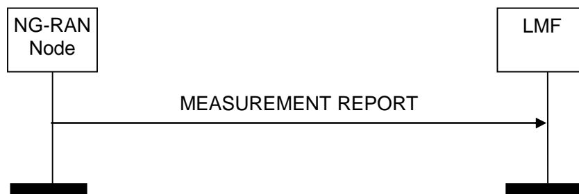
Figure 8.5.2.2.1: Measurement Report procedure. Successful operation.
