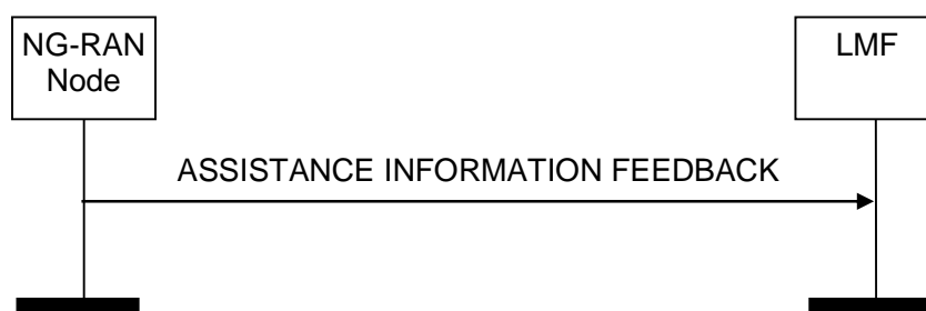
Figure 8.4.2.2-1: Assistance Information Feedback procedure
