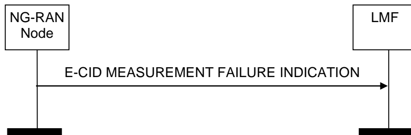
Figure 8.2.2.2-1: E-CID Measurement Failure Indication, successful operation
