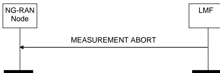
Figure 8.5.4.2.1: Measurement Abort Procedure: Successful Operation.
