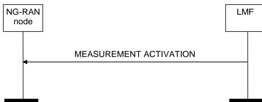
Figure 8.2.13.2-1: Measurement Activation procedure, successful operation
