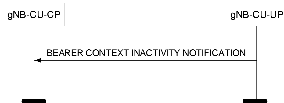
Figure 8.3.6.2-1: Bearer Context Inactivity Notification procedure: Successful Operation.
