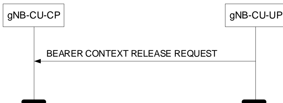
Figure 8.3.5.2-1: Bearer Context Release Request procedure: Successful Operation.
