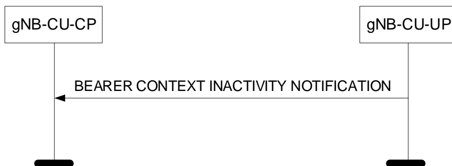
Figure 8.3.6.2-1: Bearer Context Inactivity Notification procedure: Successful Operation.
