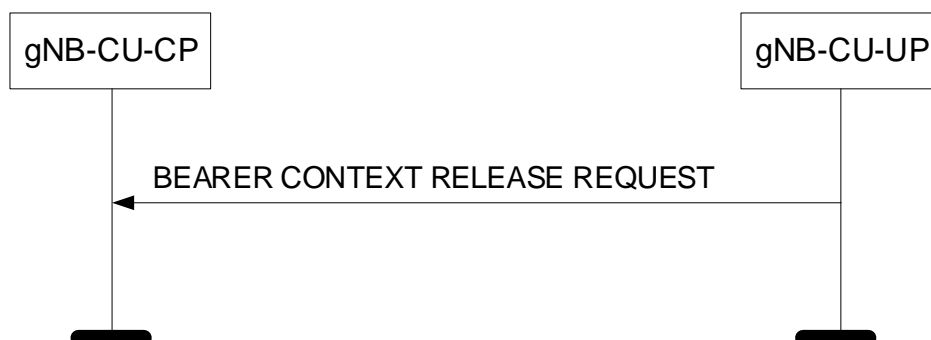
Figure 8.3.5.2-1: Bearer Context Release Request procedure: Successful Operation.
