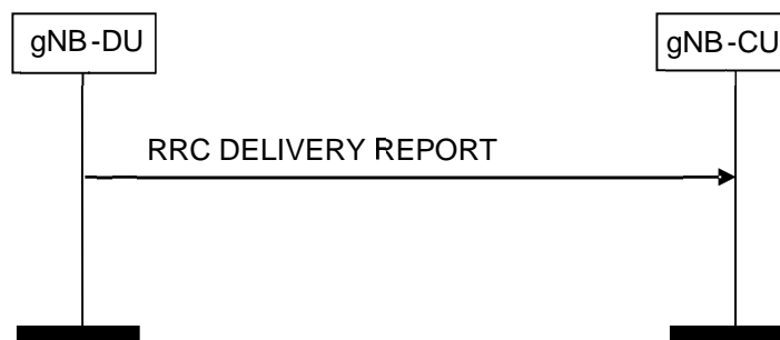
Figure 8.4.4.2-1: RRC Delivery Report procedure.
