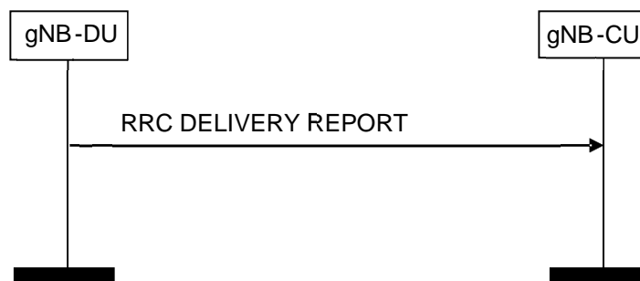
Figure 8.4.4.2-1: RRC Delivery Report procedure.
