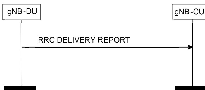
Figure 8.4.4.2-1: RRC Delivery Report procedure.
