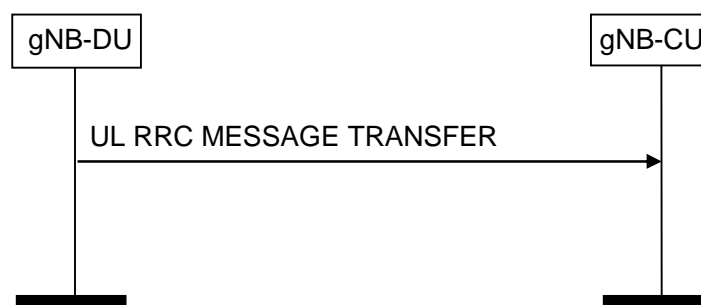
Figure 8.4.3.2-1: UL RRC Message Transfer procedure
