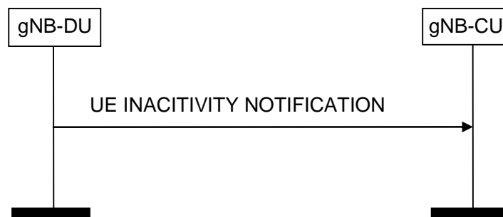
Figure 8.3.6.2-1: UE Inactivity Notification procedure.
