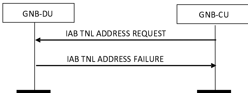
Figure 8.10.3.3-1: IAB TNL Address Allocation procedure: Unsuccessful Operation
