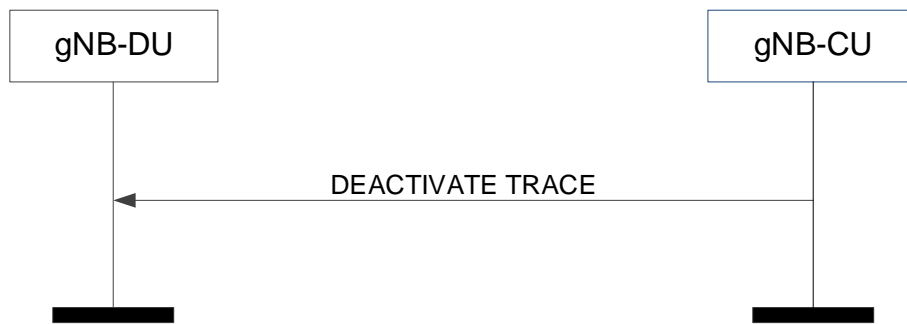
Figure 8.8.2.2-1: Deactivate trace procedure: Successful Operation
