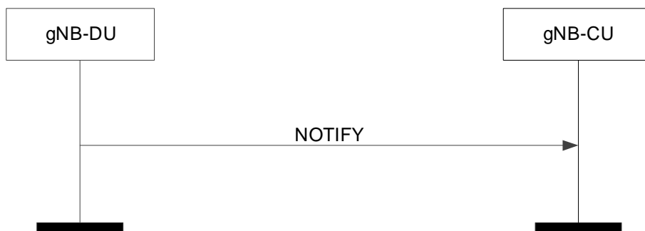
Figure 8.3.7.2-1: Notify procedure. Successful operation.
