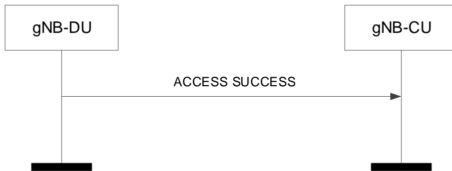
Figure 8.3.8.2-1: Access Success procedure. Successful operation.
