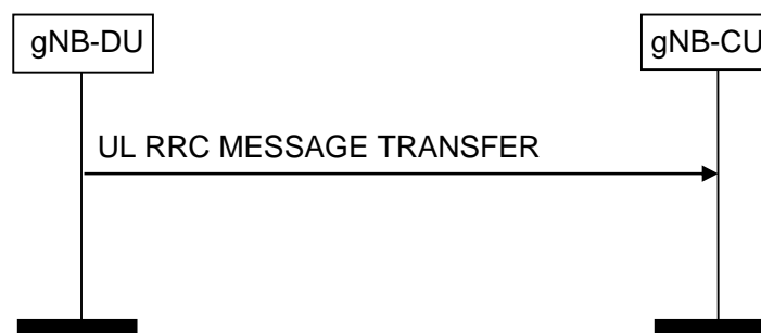
Figure 8.4.3.2-1: UL RRC Message Transfer procedure
