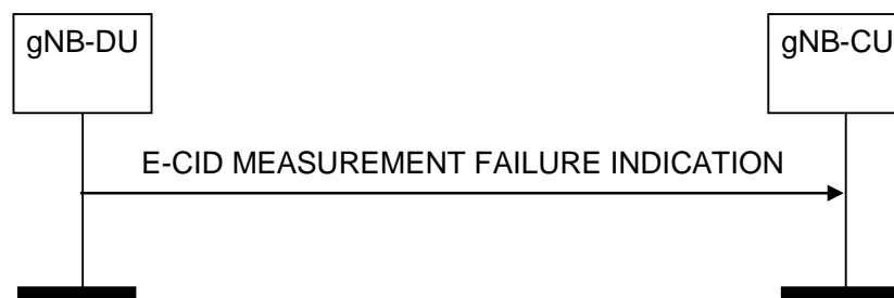
Figure 8.13.13.2-1: E-CID Measurement Failure Indication, successful operation
