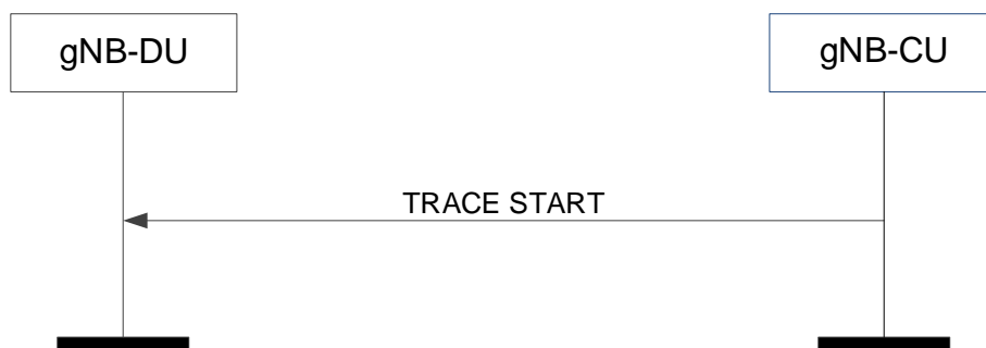
Figure 8.8.1.2-1: Trace start procedure: Successful Operation.
