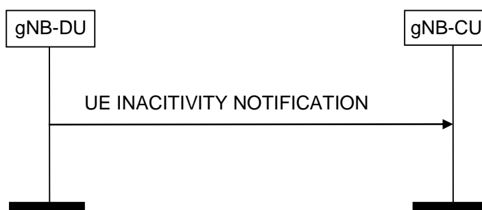
Figure 8.3.6.2-1: UE Inactivity Notification procedure.
