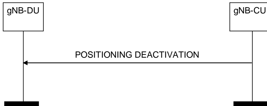
Figure 8.13.11.2-1: Positioning Deactivation procedure, successful operation
