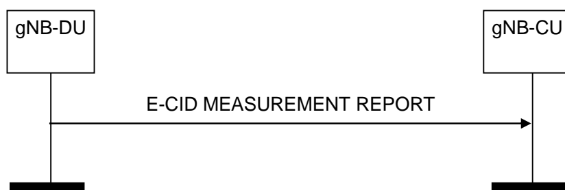
Figure 8.13.14.2-1: E-CID Measurement Report procedure, successful operation
