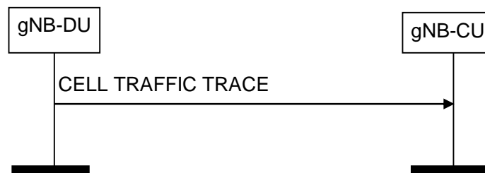
Figure 8.8.3.2-1: Cell Traffic Trace procedure. Successful operation.
