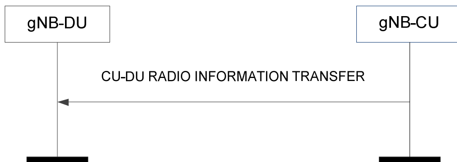
Figure 8.9.2.2-1: CU-DU Radio Information Transfer procedure.
