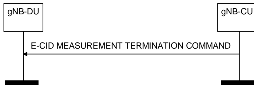
Figure 8.13.15.2-1: E-CID Measurement Termination procedure, successful operation
