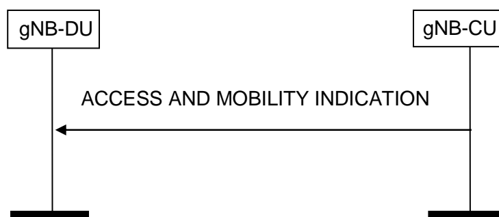
Figure 8.11.1.2-1: Access and Mobility Indication procedure. Successful operation
