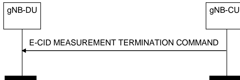
Figure 8.13.15.2-1: E-CID Measurement Termination procedure, successful operation
