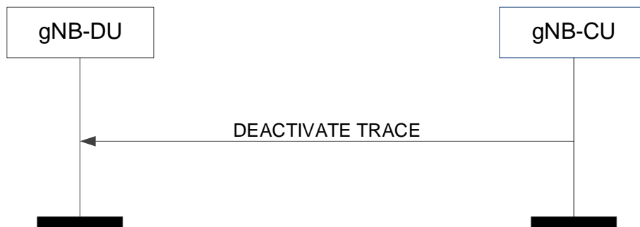
Figure 8.8.2.2-1: Deactivate trace procedure: Successful Operation
