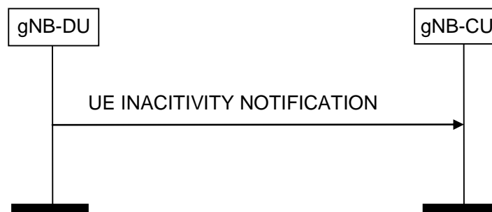
Figure 8.3.6.2-1: UE Inactivity Notification procedure.
