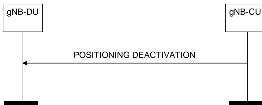
Figure 8.13.11.2-1: Positioning Deactivation procedure, successful operation
