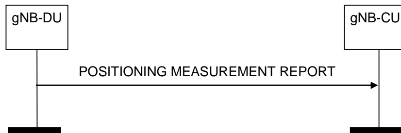
Figure 8.13.4.2-1: Positioning Measurement Report procedure: successful operation
