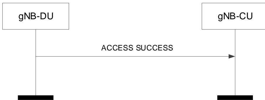
Figure 8.3.8.2-1: Access Success procedure. Successful operation.
