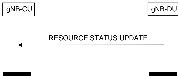
Figure 8.2.11.2-1: Resource Status Reporting, successful operation
