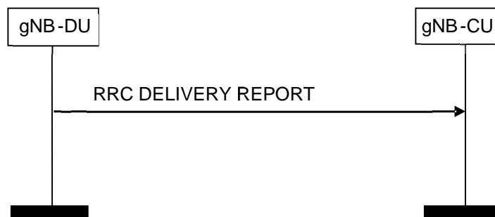
Figure 8.4.4.2-1: RRC Delivery Report procedure.
