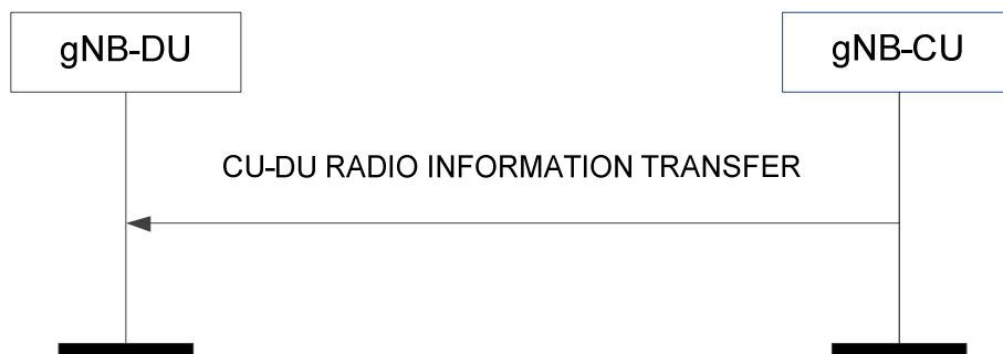
Figure 8.9.2.2-1: CU-DU Radio Information Transfer procedure.
