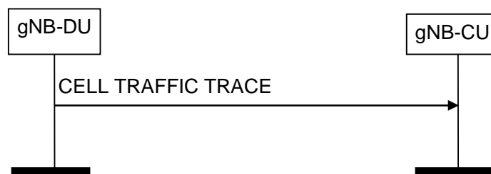
Figure 8.8.3.2-1: Cell Traffic Trace procedure. Successful operation.
