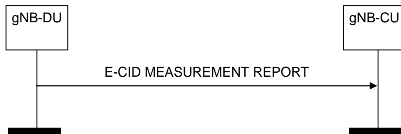
Figure 8.13.14.2-1: E-CID Measurement Report procedure, successful operation
