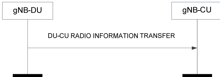
Figure 8.9.1.2-1: DU-CU Radio Information Transfer procedure.
