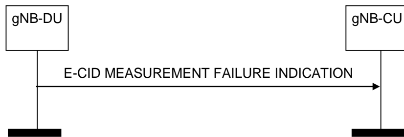
Figure 8.13.13.2-1: E-CID Measurement Failure Indication, successful operation
