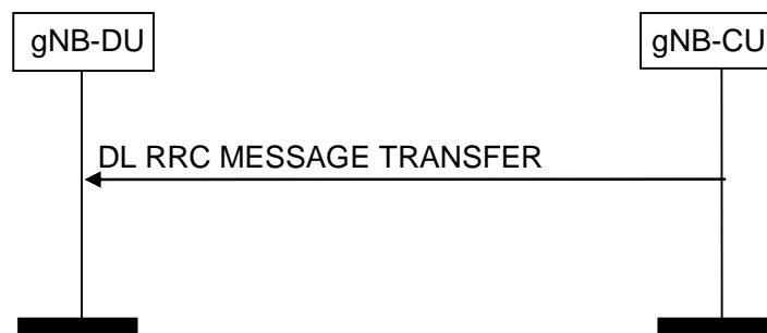
Figure 8.4.2.2-1: DL RRC Message Transfer procedure
