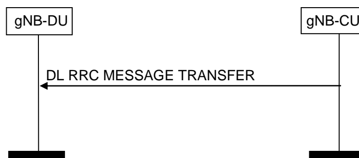
Figure 8.4.2.2-1: DL RRC Message Transfer procedure
