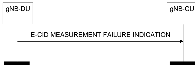
Figure 8.13.13.2-1: E-CID Measurement Failure Indication, successful operation
