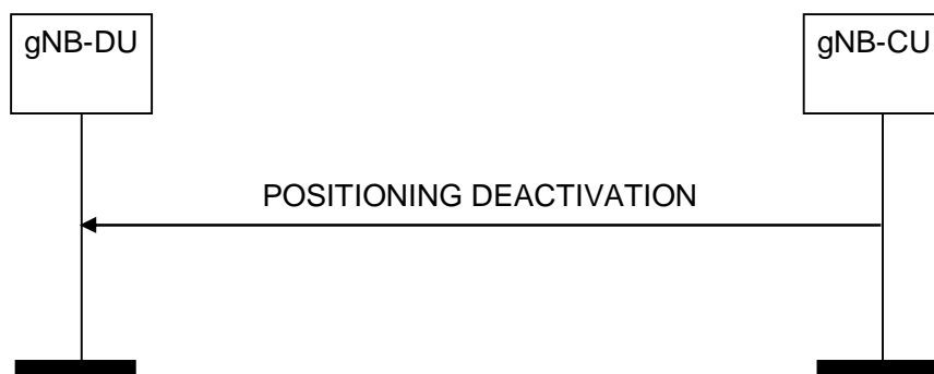
Figure 8.13.11.2-1: Positioning Deactivation procedure, successful operation
