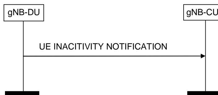
Figure 8.3.6.2-1: UE Inactivity Notification procedure.
