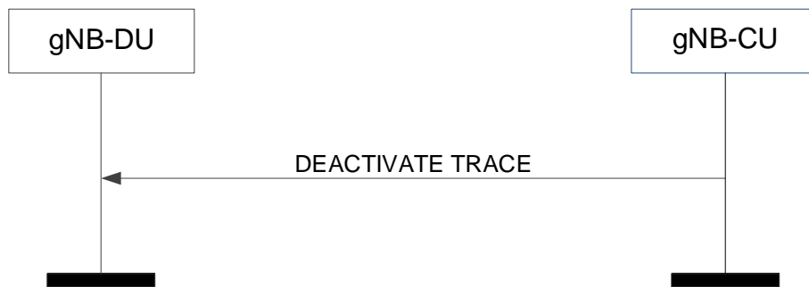
Figure 8.8.2.2-1: Deactivate trace procedure: Successful Operation
