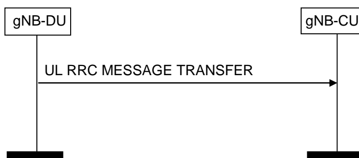
Figure 8.4.3.2-1: UL RRC Message Transfer procedure
