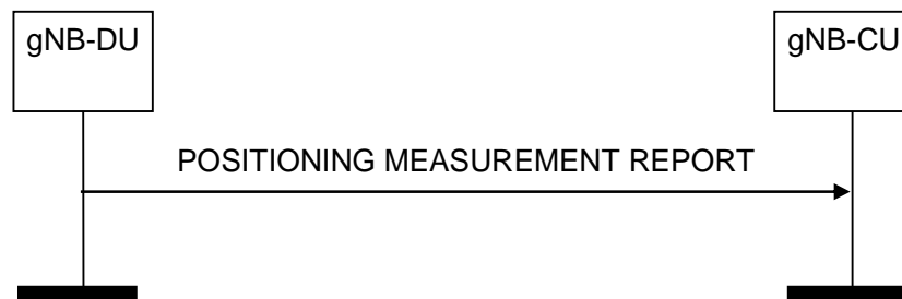
Figure 8.13.4.2-1: Positioning Measurement Report procedure: successful operation
