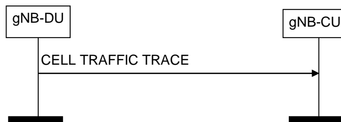
Figure 8.8.3.2-1: Cell Traffic Trace procedure. Successful operation.
