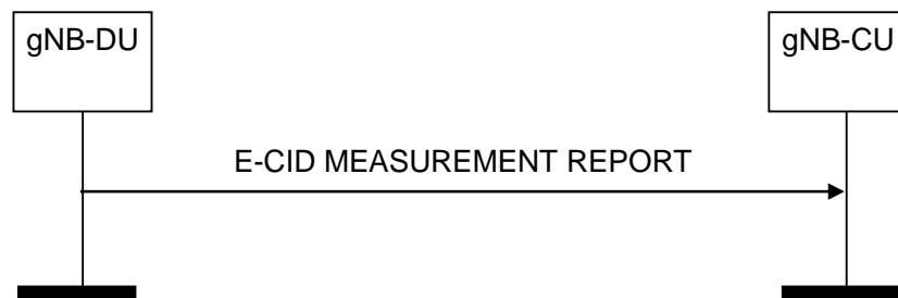
Figure 8.13.14.2-1: E-CID Measurement Report procedure, successful operation
