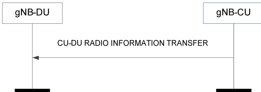
Figure 8.9.2.2-1: CU-DU Radio Information Transfer procedure.
