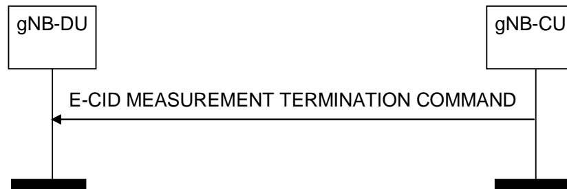
Figure 8.13.15.2-1: E-CID Measurement Termination procedure, successful operation
