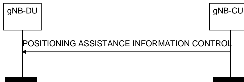
Figure 8.13.1.2-1: Positioning Assistance Information Control procedure
