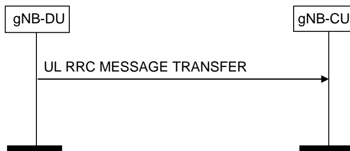
Figure 8.4.3.2-1: UL RRC Message Transfer procedure
