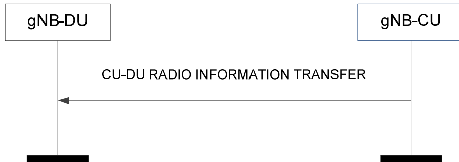
Figure 8.9.2.2-1: CU-DU Radio Information Transfer procedure.
