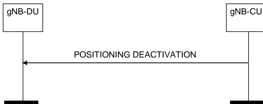
Figure 8.13.11.2-1: Positioning Deactivation procedure, successful operation
