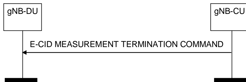
Figure 8.13.15.2-1: E-CID Measurement Termination procedure, successful operation
