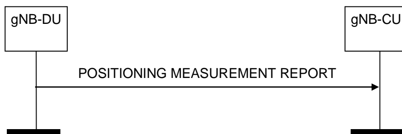
Figure 8.13.4.2-1: Positioning Measurement Report procedure: successful operation
