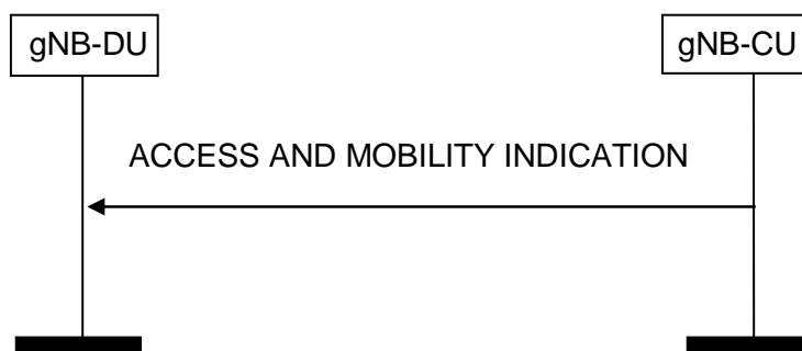
Figure 8.11.1.2-1: Access and Mobility Indication procedure. Successful operation
