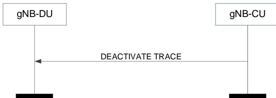
Figure 8.8.2.2-1: Deactivate trace procedure: Successful Operation
