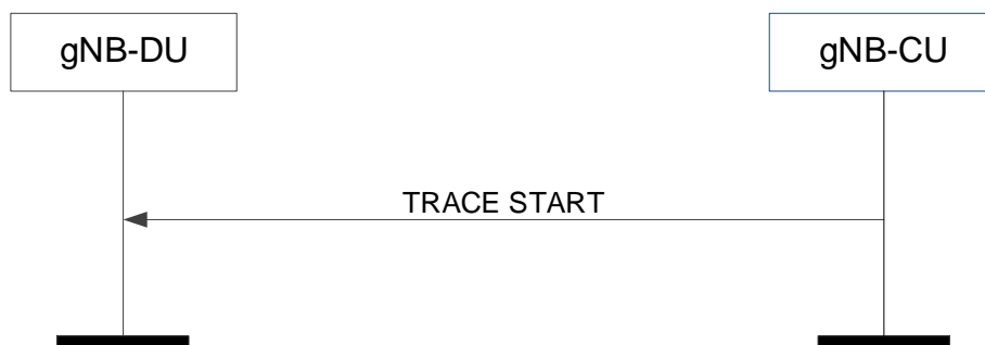
Figure 8.8.1.2-1: Trace start procedure: Successful Operation.
