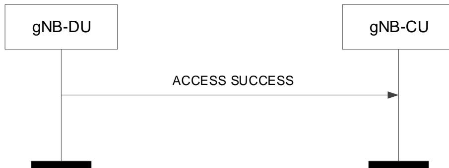
Figure 8.3.8.2-1: Access Success procedure. Successful operation.
