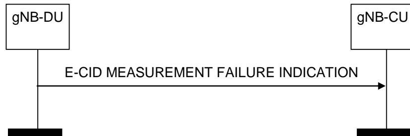
Figure 8.13.13.2-1: E-CID Measurement Failure Indication, successful operation
