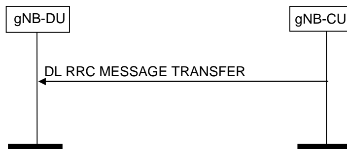
Figure 8.4.2.2-1: DL RRC Message Transfer procedure
