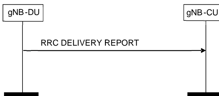
Figure 8.4.4.2-1: RRC Delivery Report procedure.
