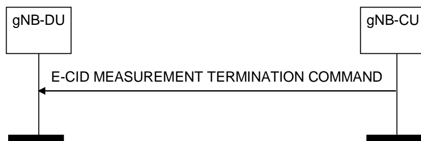
Figure 8.13.15.2-1: E-CID Measurement Termination procedure, successful operation
