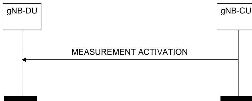
Figure 8.13.19.2-1: Measurement Activation procedure, successful operation
