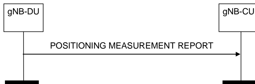
Figure 8.13.4.2-1: Positioning Measurement Report procedure: successful operation
