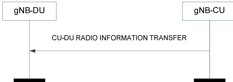
Figure 8.9.2.2-1: CU-DU Radio Information Transfer procedure.
