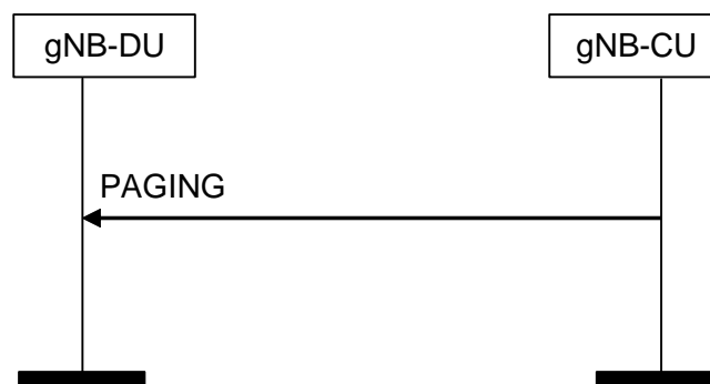
Figure 8.7.1.2-1: Paging procedure. Successful operation.
