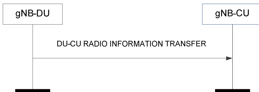
Figure 8.9.1.2-1: DU-CU Radio Information Transfer procedure.
