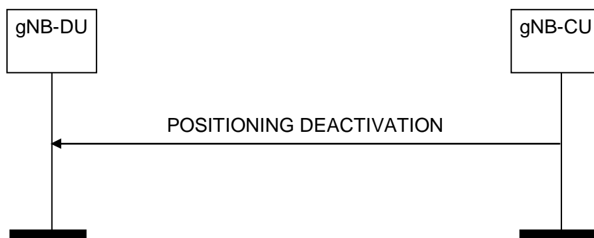
Figure 8.13.11.2-1: Positioning Deactivation procedure, successful operation
