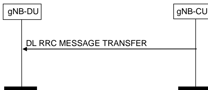
Figure 8.4.2.2-1: DL RRC Message Transfer procedure
