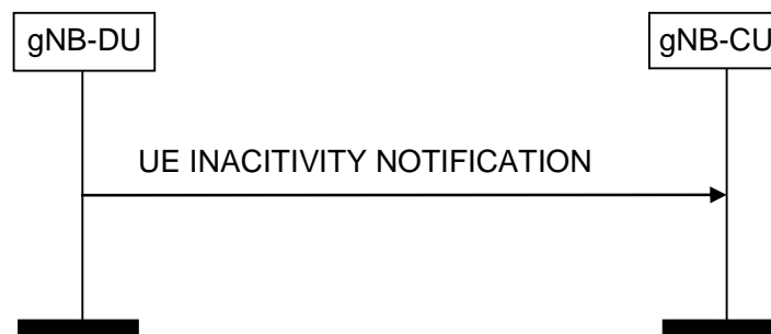
Figure 8.3.6.2-1: UE Inactivity Notification procedure.
