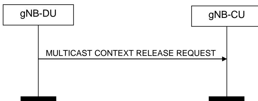
Figure 8.14.8.2-1: Multicast Context Release Request procedure. Successful operation
