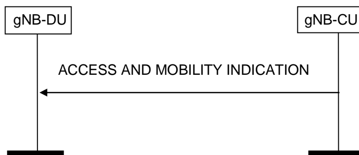
Figure 8.11.1.2-1: Access and Mobility Indication procedure. Successful operation
