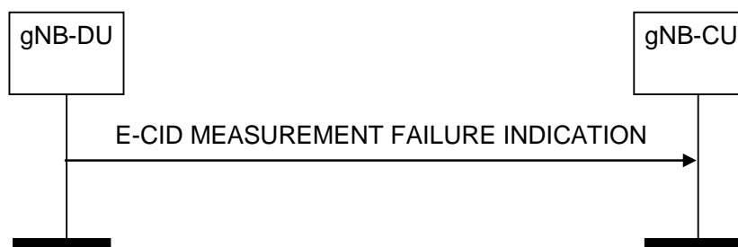
Figure 8.13.13.2-1: E-CID Measurement Failure Indication, successful operation
