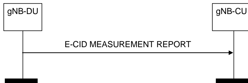
Figure 8.13.14.2-1: E-CID Measurement Report procedure, successful operation
