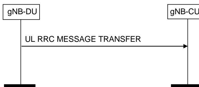
Figure 8.4.3.2-1: UL RRC Message Transfer procedure
