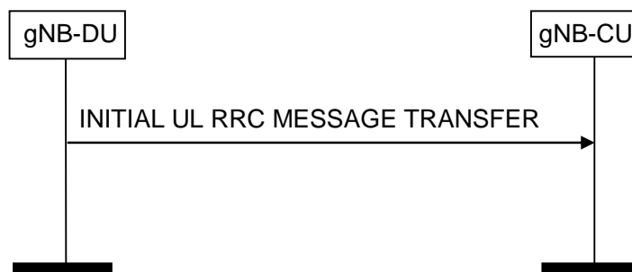
Figure 8.4.1.2-1: Initial UL RRC Message Transfer procedure.
