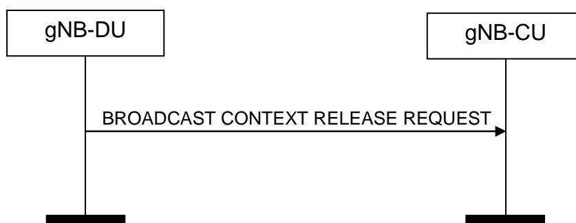
Figure 8.14.3.2-1: Broadcast Context Release Request procedure. Successful operation
