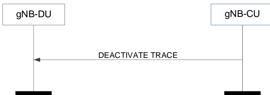
Figure 8.8.2.2-1: Deactivate trace procedure: Successful Operation
