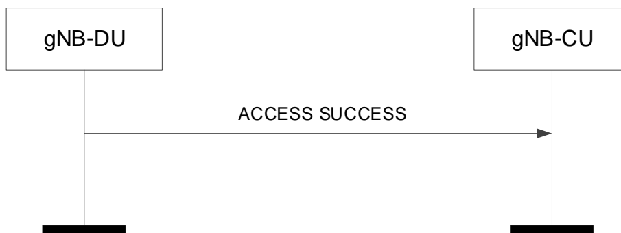
Figure 8.3.8.2-1: Access Success procedure. Successful operation.
