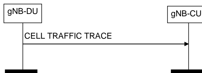
Figure 8.8.3.2-1: Cell Traffic Trace procedure. Successful operation.
