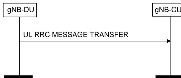
Figure 8.4.3.2-1: UL RRC Message Transfer procedure
