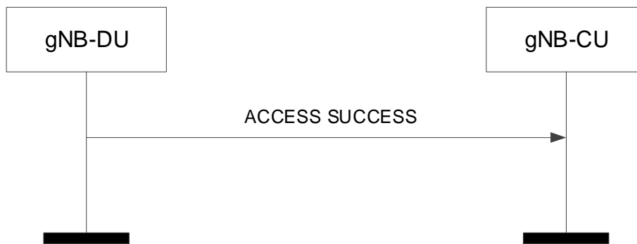
Figure 8.3.8.2-1: Access Success procedure. Successful operation.
