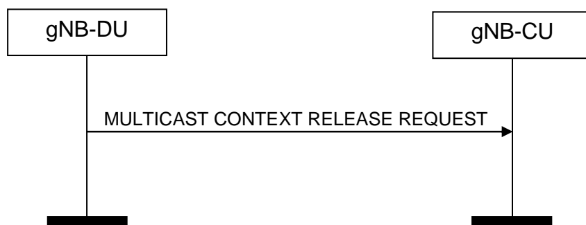
Figure 8.14.8.2-1: Multicast Context Release Request procedure. Successful operation
