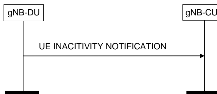
Figure 8.3.6.2-1: UE Inactivity Notification procedure.
