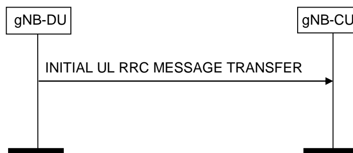
Figure 8.4.1.2-1: Initial UL RRC Message Transfer procedure.
