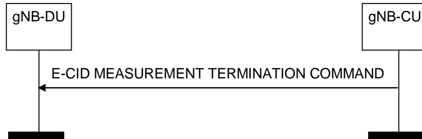
Figure 8.13.15.2-1: E-CID Measurement Termination procedure, successful operation
