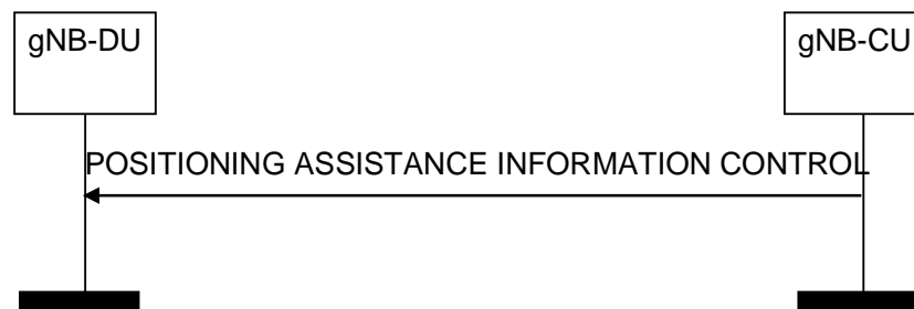
Figure 8.13.1.2-1: Positioning Assistance Information Control procedure
