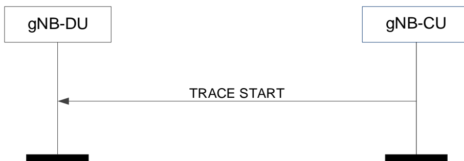
Figure 8.8.1.2-1: Trace start procedure: Successful Operation.
