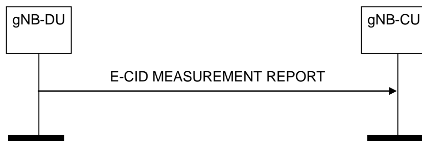
Figure 8.13.14.2-1: E-CID Measurement Report procedure, successful operation
