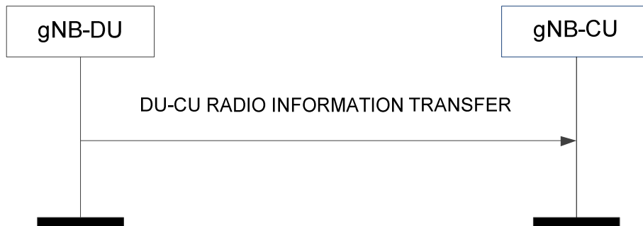
Figure 8.9.1.2-1: DU-CU Radio Information Transfer procedure.
