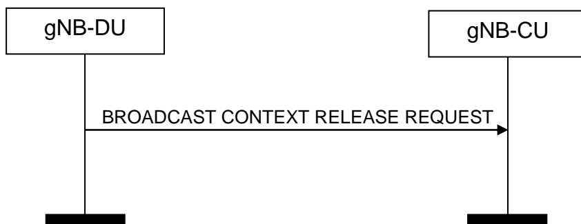
Figure 8.14.3.2-1: Broadcast Context Release Request procedure. Successful operation
