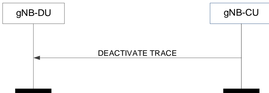
Figure 8.8.2.2-1: Deactivate trace procedure: Successful Operation
