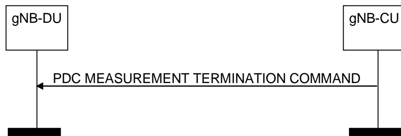
Figure 8.15.3.2-1: PDC Measurement Termination procedure: successful operation
