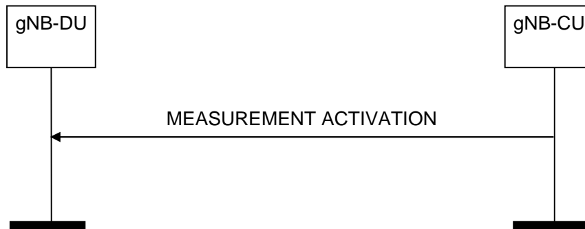
Figure 8.13.19.2-1: Measurement Activation procedure, successful operation
