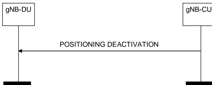
Figure 8.13.11.2-1: Positioning Deactivation procedure, successful operation
