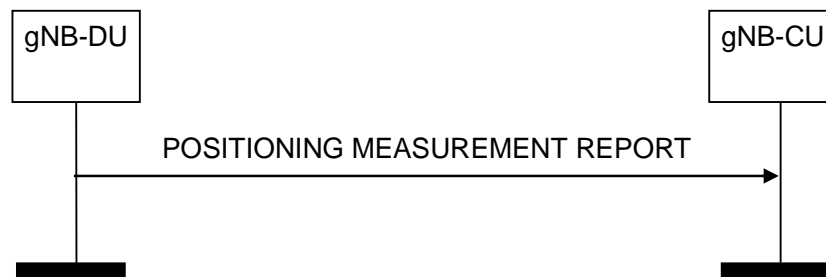
Figure 8.13.4.2-1: Positioning Measurement Report procedure: successful operation
