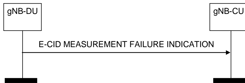
Figure 8.13.13.2-1: E-CID Measurement Failure Indication, successful operation
