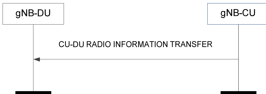
Figure 8.9.2.2-1: CU-DU Radio Information Transfer procedure.
