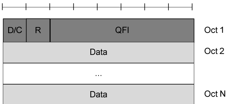
Figure 6.2.2.3-1: UL SDAP Data PDU format with SDAP header
