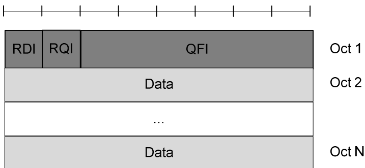
Figure 6.2.2.2-1: DL SDAP Data PDU format with SDAP header
