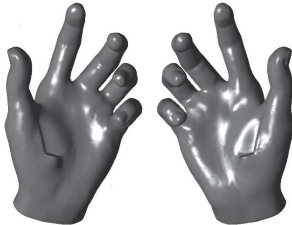
Figure B.2.3-1 Wide Grip hand (© 2001 – 2022 CTIA Certification. Reproduced with permission.), defined in the CTIA Certification OTA Test Plan
