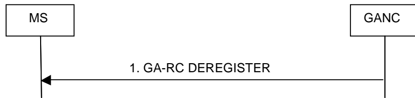
Figure 13: De-Registration initiated by the GANC
