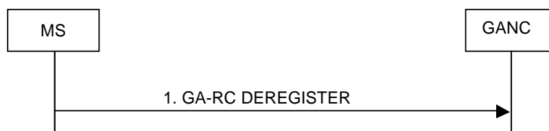
Figure 12: De-Registration initiated by the MS
