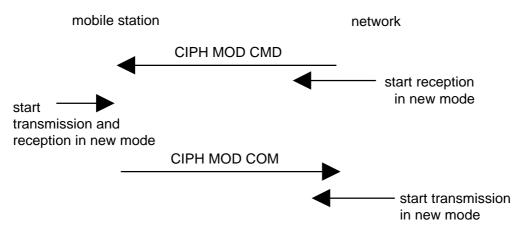
Figure 3.4.7.2.1: Ciphering mode setting sequence
