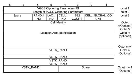
Figure 10.5.2.42b.1: VGCS Ciphering Parameters Information Element
