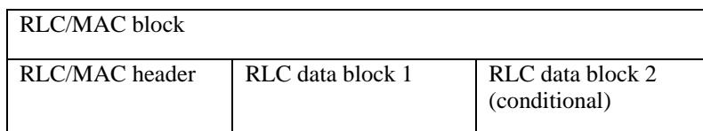
**Figure 10.0a.2.1: RLC/MAC block structure for EGPRS data transfer (FANR not activated)**
