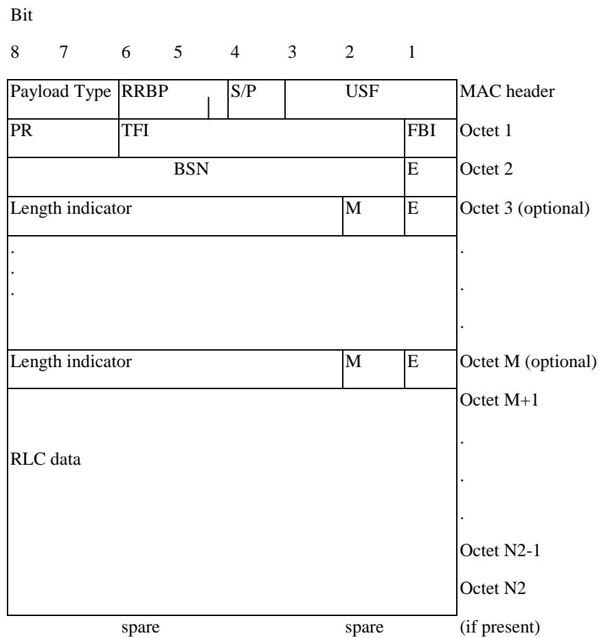
**Figure 10.2.1.1: Downlink RLC data block with MAC header**
