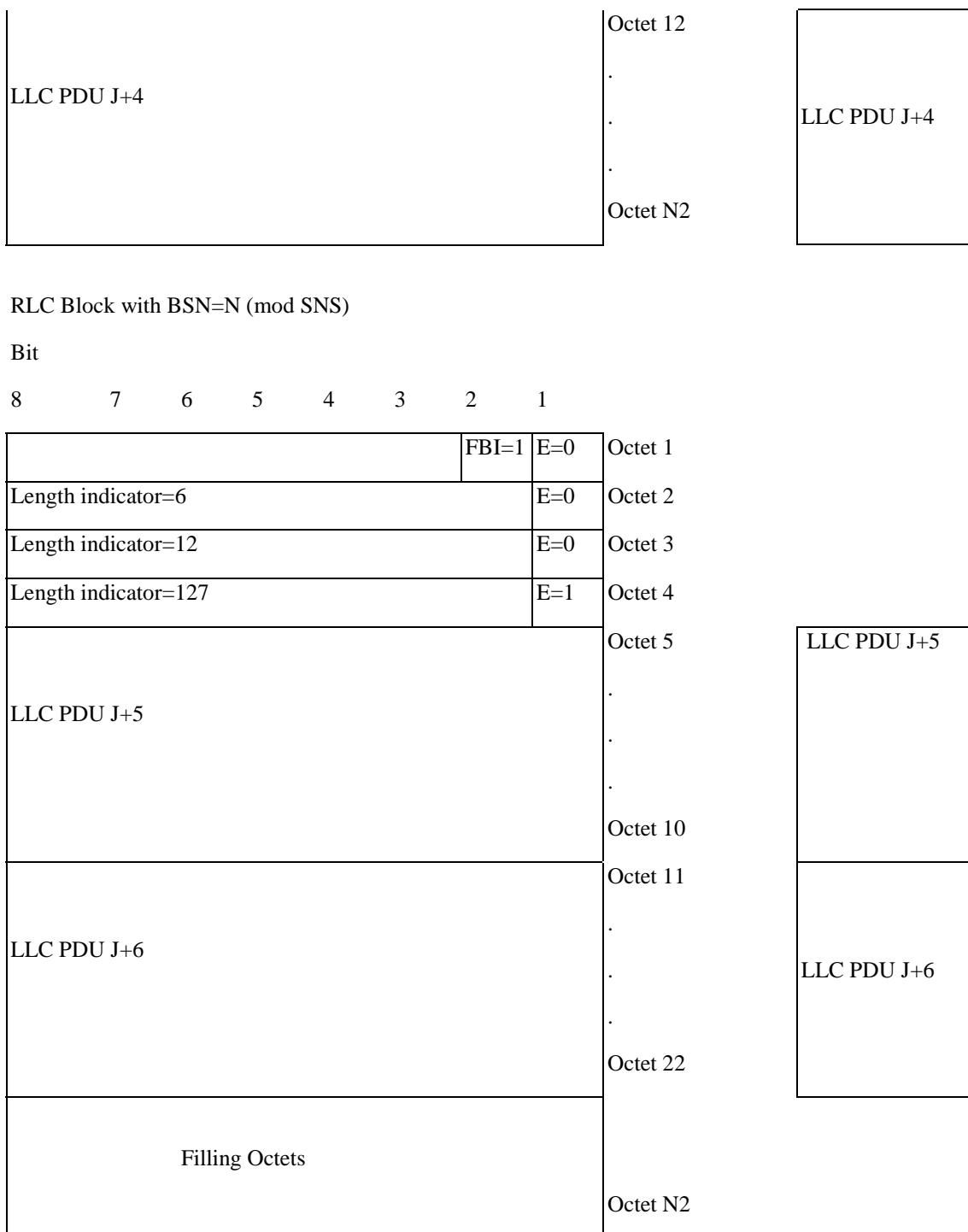
**Figure B.9: Example for the case when the LLC PDU fills exactly the RLC data block (LLC PDU J+2 and LLC PDU J+4) and when the last LLC PDU cannot not fill the last RLC data block(LLC PDU J+6)**
