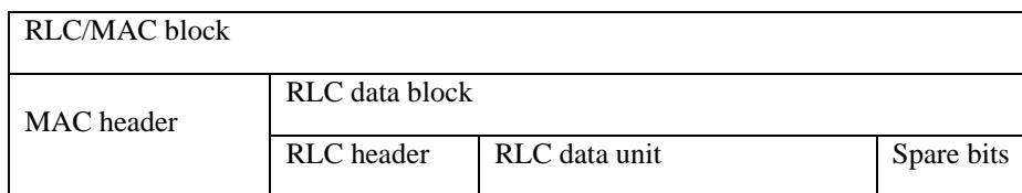
**Figure 10.0a.1.1: RLC/MAC block structure for data transfer for GPRS**
