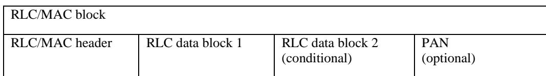
**Figure 10.0a.2.2: RLC/MAC block structure for EGPRS data transfer (FANR activated)**
