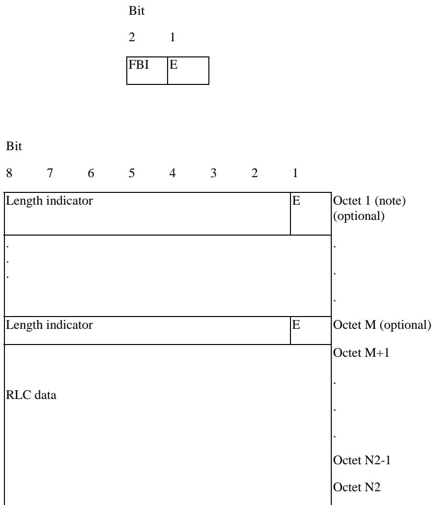
NOTE: If padding is used, then "Octet 1" shall be replaced by "Octet 7", see example in annex J.
