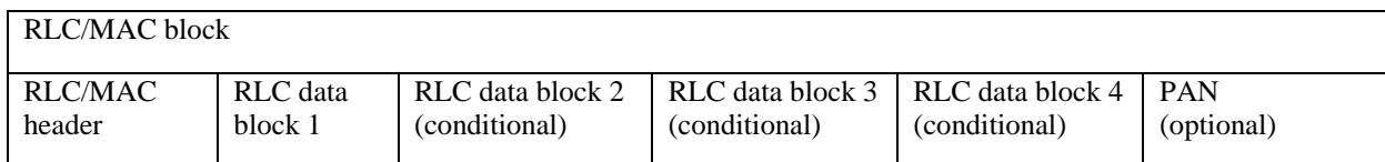
**Figure 10.0a.2.3: RLC/MAC block structure for EGPRS2 data transfer**
