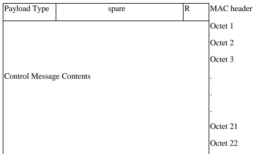
**Figure 10.3.2.1: Uplink RLC/MAC control block together with its MAC header**
