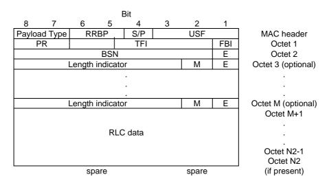
Figure 10.2.1.1: Downlink RLC data block with MAC header
