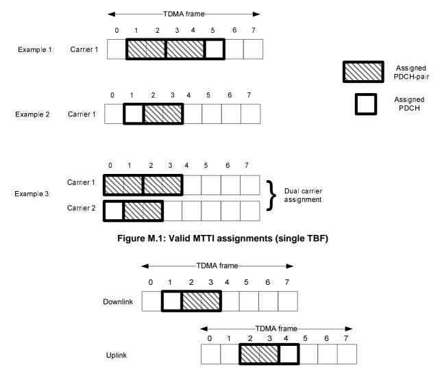
Figure M.2: Valid MTTI assignment (1 uplink TBF & 1 downlink TBF)
