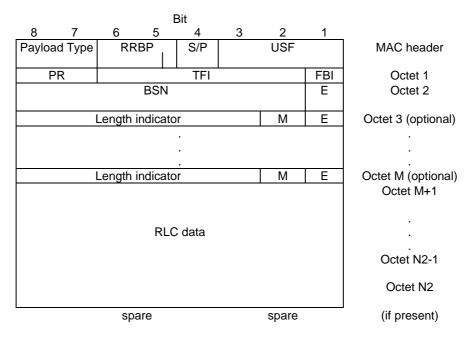
Figure 10.2.1.1: Downlink RLC data block with MAC header
