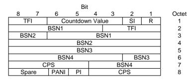
Figure 10.3a.4.9.1: Combined uplink RLC data block header for UBS-11, UBS-12.
