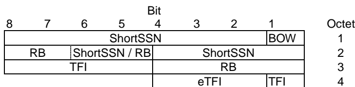
Figure 10.3a.5.2: Uplink Piggy-backed Ack/Nack field (SSN-based, eTFI assigned)
