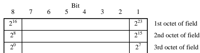
Figure 6: FCS mapping convention
