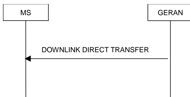
Figure 7.17.2.1/3GPP TS 44.118: Downlink Direct transfer, normal flow
