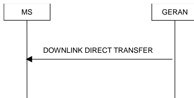
Figure 7.17.2.1: Downlink Direct transfer, normal flow
