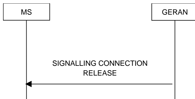
Figure 7.15.1.1.1: Signalling Connection Release procedure, normal case
