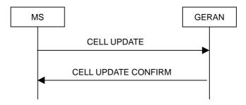
Figure 7.8.1.1: Cell Update procedure, basic flow
