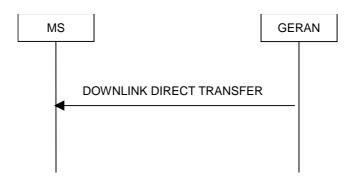
Figure 7.17.2.1: Downlink Direct transfer, normal flow
