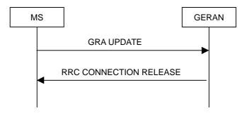
Figure 7.8.1.8: GRA Update procedure, failure case
