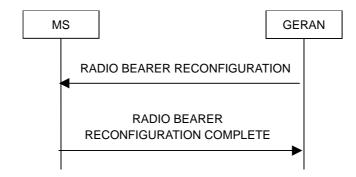
Figure 7.14.1.3: Radio Bearer Reconfiguration, normal flow
