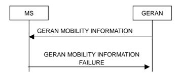
Figure 7.8.3.2: GERAN Mobility Information procedure, failure case
