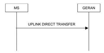
Figure 7.17.3.1: Uplink Direct transfer, normal flow
