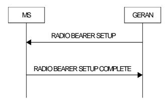
Figure 7.14.1.1: Radio Bearer Establishment, normal case
