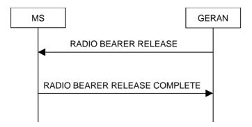
Figure 7.14.1.5: Radio Bearer Release, normal case
