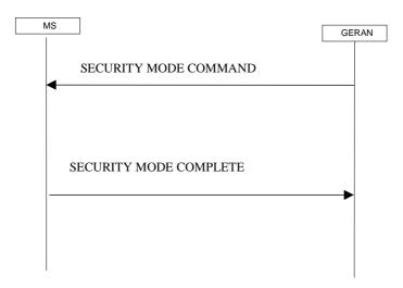
Figure 7.16.1.1: Security mode control procedure
