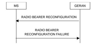
Figure 7.14.1.4: Radio Bearer Reconfiguration, failure case
