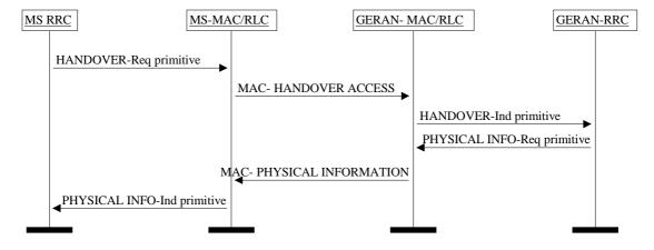
Figure 7.18.6.0.1: Handover Access procedure
