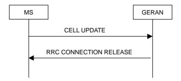
Figure 7.8.1.5: Cell Update procedure, failure case
