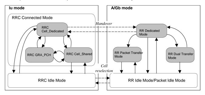
Figure 6.1.1: Transitions between RR modes of operation and RRC states and modes.
