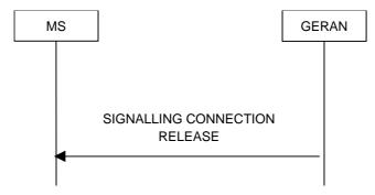
Figure 7.15.1.1.1: Signalling Connection Release procedure, normal case
