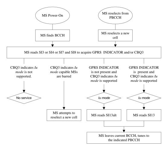
Figure 7.3.2.1: Behaviour of *lu mode* only capable MS on BCCH.
