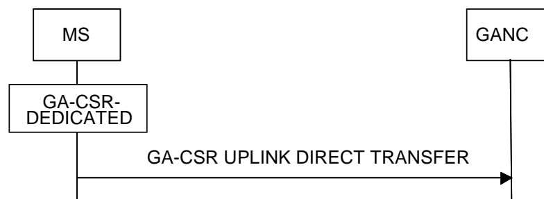
Figure 7.2.1.1 Uplink Direct Transfer, normal flow
