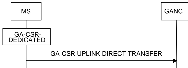
Figure 7.2.1.1 Uplink Direct Transfer, normal flow
