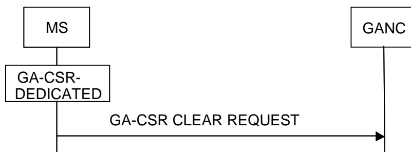
Figure 7.5.1.1 Initiation of GA-CSR connection release by MS
