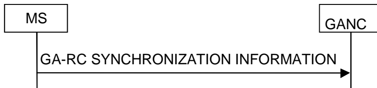
Figure 6.6.1 MS initiated synchronization procedure
