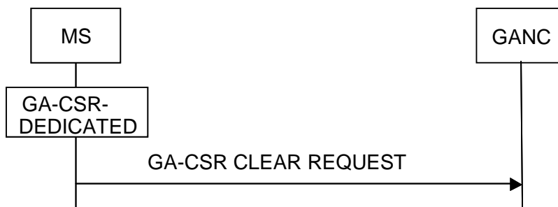
Figure 7.5.1.1 Initiation of GA-CSR connection release by MS
