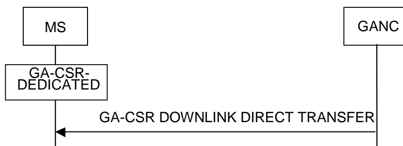
Figure 7.2.3.1 Downlink Direct Transfer, normal flow
