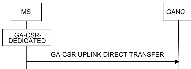
Figure 7.2.1.1 Uplink Direct Transfer, normal flow
