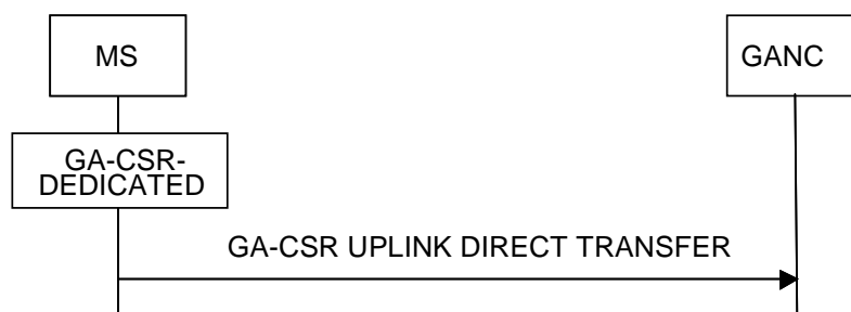
Figure 7.2.1.1 Uplink Direct Transfer, normal flow
