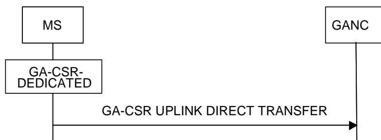
Figure 7.2.1.1 Uplink Direct Transfer, normal flow
