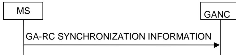
Figure 6.6.1 MS initiated synchronization procedure
