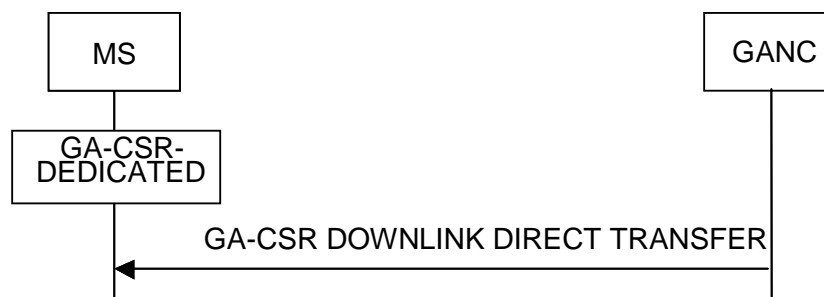
Figure 7.2.3.1 Downlink Direct Transfer, normal flow
