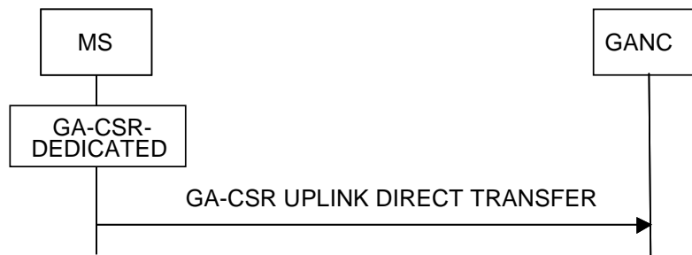
Figure 7.2.1.1 Uplink Direct Transfer, normal flow
