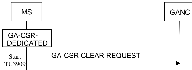
Figure 7.5.1.1 Initiation of GA-CSR connection release by MS
