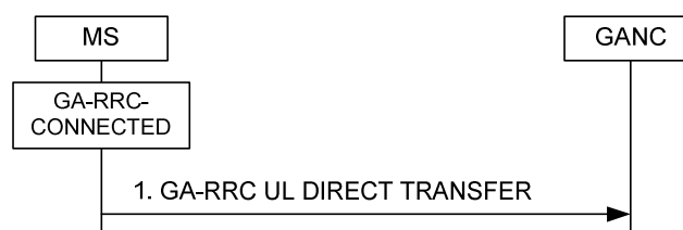
Figure 8a.2.3.1 Uplink direct transfer, normal flow
