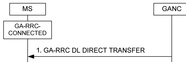
Figure 8a.2.5.1 Downlink direct transfer, normal flow
