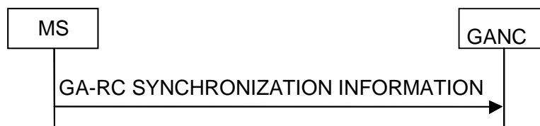
Figure 6.6.1 MS initiated synchronization procedure
