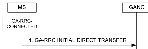
Figure 8a.2.1.1 Initial direct transfer, normal flow
