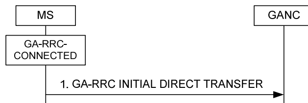
Figure 8a.2.1.1 Initial direct transfer, normal flow
