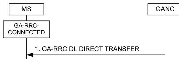
Figure 8a.2.5.1 Downlink direct transfer, normal flow
