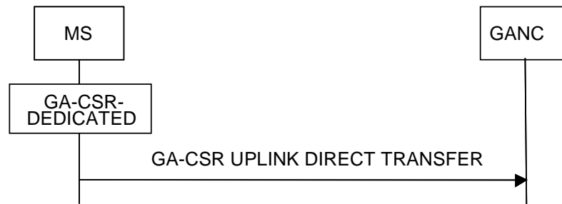
Figure 7.2.1.1 Uplink Direct Transfer, normal flow
