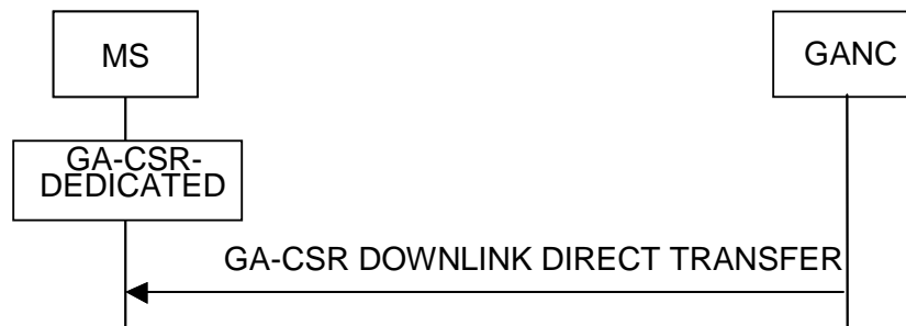
Figure 7.2.3.1 Downlink Direct Transfer, normal flow
