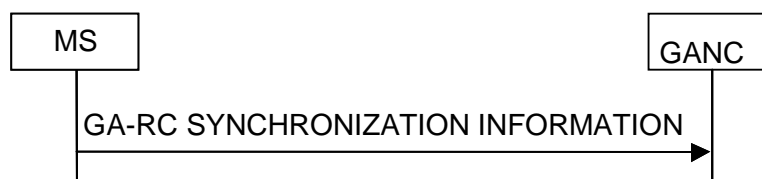
Figure 6.6.1 MS initiated synchronization procedure
