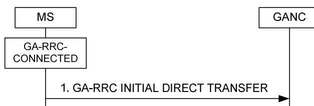
Figure 8a.2.1.1 Initial direct transfer, normal flow
