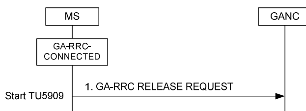
Figure 8a.5.1.1 GA-RRC connection release request by MS
