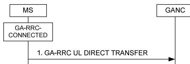
Figure 8a.2.3.1 Uplink direct transfer, normal flow
