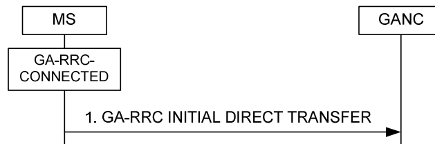
Figure 8a.2.1.1 Initial direct transfer, normal flow
