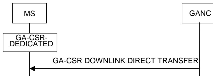
Figure 7.2.3.1 Downlink Direct Transfer, normal flow
