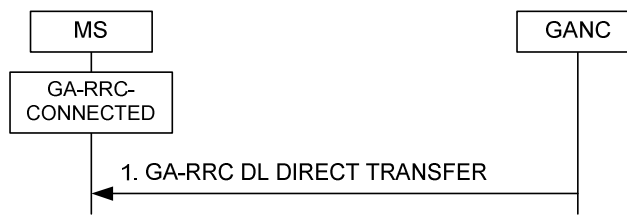
Figure 8a.2.5.1 Downlink direct transfer, normal flow
