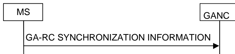
Figure 6.6.1 MS initiated synchronization procedure
