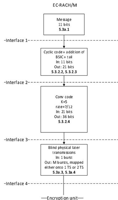
**Figure 2af: Channel Coding and Interleaving Organization for EC-RACH**
