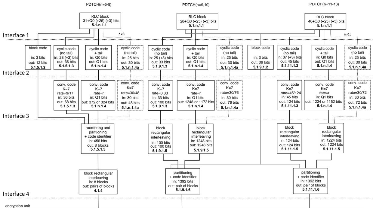
Figure 1eb: Channel Coding and Interleaving Organization for EGPRS Downlink Packet Data Channels
