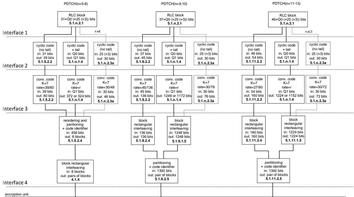
Figure 1ea: Channel Coding and Interleaving Organization for EGPRS Uplink Packet Data Channels
